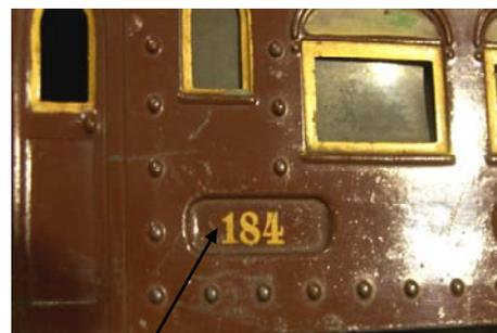
Rubber Stamped 184 and 186 (Not Shown) Instead of Plates Indentations For Plates, Tab Slots Not Cut
