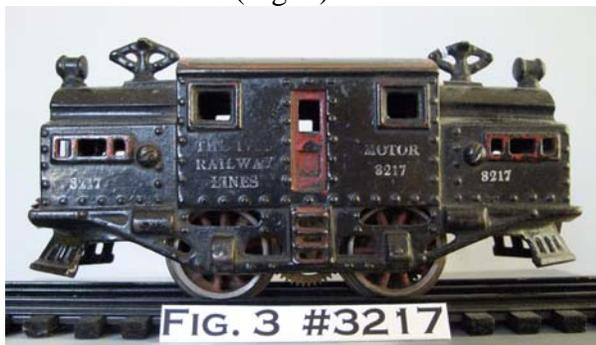
uses the 3rd casting with integral pilots and a small "ci" nub extending out from the frame above the pilot to hold the hook coupler attached by a rivet. The gears are skeletonized brass. The #3218 from 1917-18 (Fig.4)
