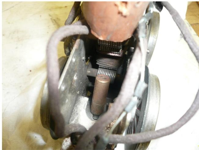
**1925 production:** Apparently realizing operational difficulties, 1925 saw the insertion of a heavy cardboard tube around which the coil was wound creating a much more rigid pathway for the central plunger to travel once the coil was energized or de-energized, and thus eliminating plunger jams caused by tearing paper; the cardboard tube did not solve the devastating functional effects of moisture damage described above.
