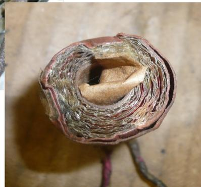
Other observations reveal moisture damage distorting the coil resulting in a badly rusted and frozen plunger. In the original patent, Sparks calls what I am referring to as a plunger, as " the movable electromagnet component or armature". ( see pictures below)
