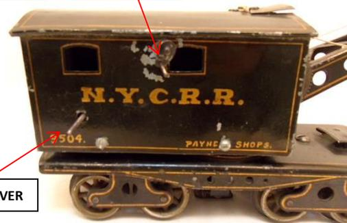
an axle mounted gear on the top of the motor to raise and lower the crane's hook, and on the same side, the reversing lever protrudes. Mr. Mizell believes he purchased the car from a local Denver collector who bought it at a York TCA meet, many years ago. The craftsmanship is too factory-like to have been built by a youngster, who might have been given a Struckiron Erector Set as a toy gift.
