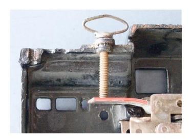
These holes were tapped for the bolt. After the body halves were bolted together the lamps were screwed into the holes and the wire passed into the body through the second hole behind the socket (Fig. 4).
