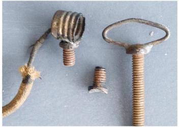
The bolt was fluxed, heated, solder applied, and the socket, also fluxed, mated onto the bolt. Both body halves had small cast in half boxes with half holes at top front and rear (Fig. 3).
