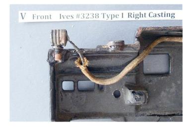
Second: there were only two subassemblies; a two-part, cast-iron body unit and a motor, wheels, pony truck and pilot unit. By attaching the pony trucks to the motor the arc of play was greater than if they had attempted to attach the trucks directly to the body (Fig. 5); Clever design!
